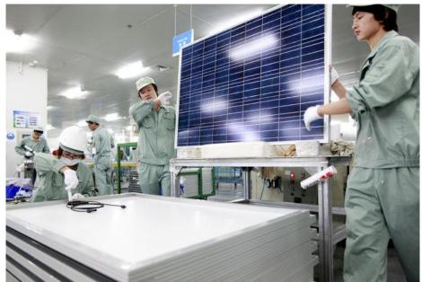
Employees assemble photovoltaic panels at Suntech Power Holdings Co.'s factory in Wuxi, Jiangsu Province, China. (Goossens)
